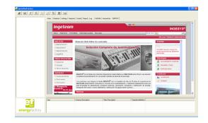
Using emulationFactory, you can emulate the behavior of any device using its CID configuration file. emulationFactory lets you modify data values, qualities etc. by sending reports or goose messages according to the configuration.
