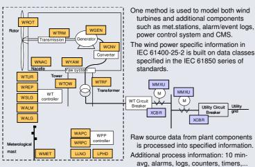
IEC 61400-25-4 specifies multiple mappings to communication profiles, where the choice depends on the functionality needed and the location of the interface;
